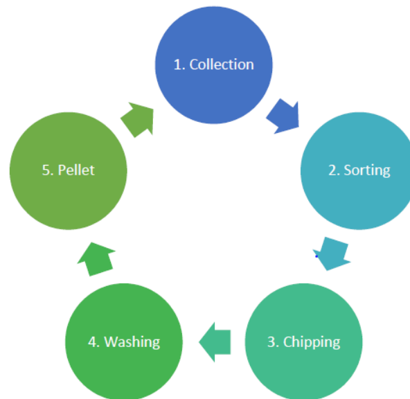
Figure 15 Plastics recycling process (adapted from Technavio, 2016 & from CSIRO, 2017)
