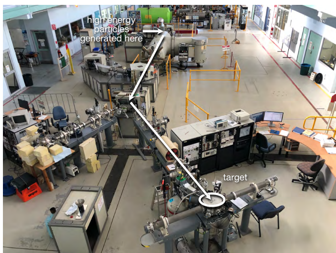
Figure 6 - The STAR accelerator generates a beam of fast particles aimed at samples in the target chamber (shown on the right). The automation of handling many packaging samples makes this an efficient system for measuring the total fluorine concentrations in large numbers of food packaging samples.
