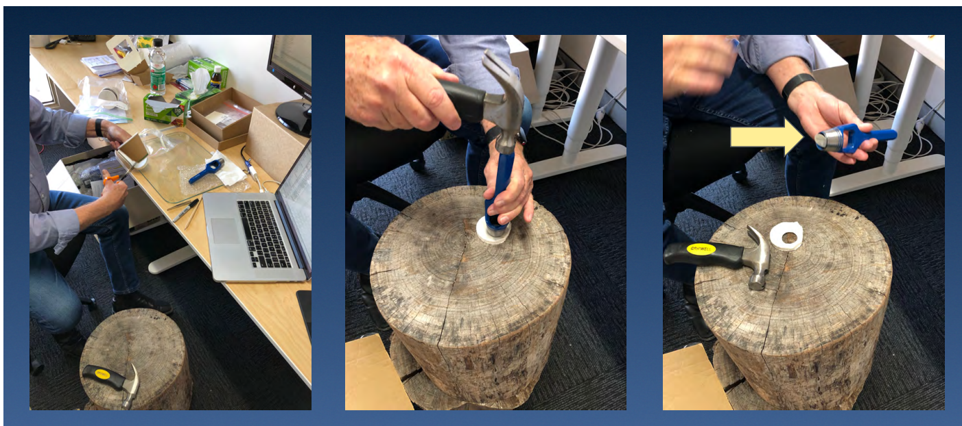
Figure 4 - Discs were removed in duplicate, near to one another on the packaging surface, and both stored in the same labelled, sealed plastic bag.
