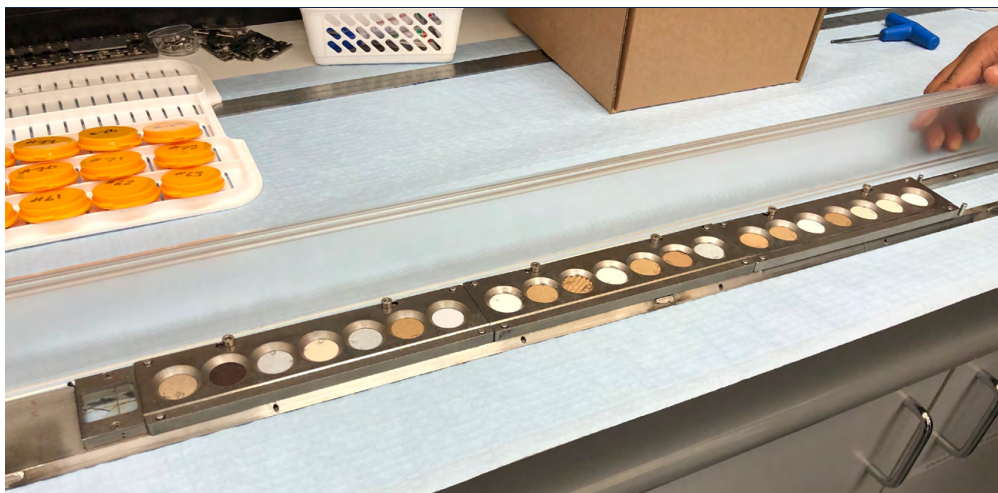
Figure 5 - The sample discs were loaded into a metal carousel that was automatically programmed to move into a target chamber to be bombarded by high-energy particles.
